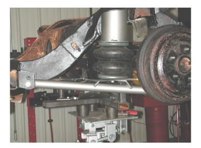
2. Fasten the lower StrongArms to the frame and axle using the  $5/8^{\circ} \times 3^{1/2^{\circ}}$  bolt and Nylok nuts supplied.
