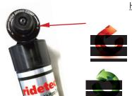
High speed compression adjustment is what is typically felt during street driving.
