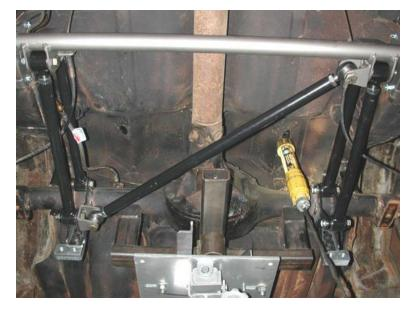
17. Bolt the lower Shockwave mount to the axle bracket using the  $\frac{1}{2}$ "-20" x 3/4" Hex Head Bolt. Apply anti-seize to the threads. It is easier to remove the bars to install these bolts.
