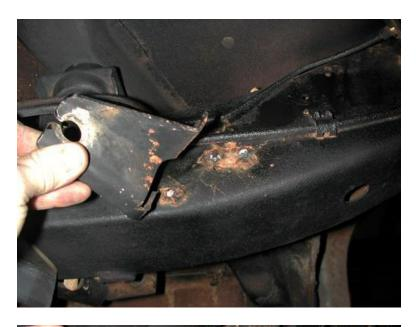
3. The parking brake brackets will be in the way of the 4 link and must be removed. Loosen the parking brake adjustment nut and remove the cable from the frame bracket. The tack weld can be broke loose with a hammer and chisel. Grind the remains of the weld smooth.
