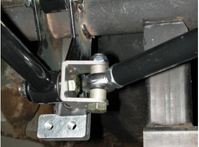
19. Insert the R-Joint spacers into the R-joint with the small OD inserted into the R-Joint center pivot. Bolt the diagonal link into place using a 5/8" x 2 3/4" bolt and nylok. It should measure 30 1/4" C-C.
