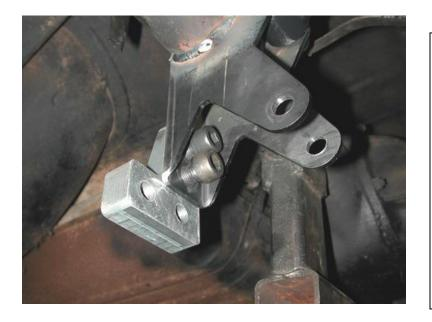
15. Swing the axle bracket up to the axle. These brackets must be centered and aligned with the crossmember mounts before welding. The brackets should be 31 5/8" apart on the outside measurement. Then just center it between the axle flanges.
