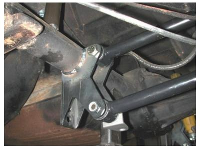
13. Insert the R-Joint spacers into the Rjoint with the small OD inserted into the R-Joint center pivot. Install the 4 link bars into the crossmember and axle bracket. Use the 5/8" x 2 3/4" bolts and nyloks supplied. Check the length of the bars; they should be 18 1/2" C-C.
