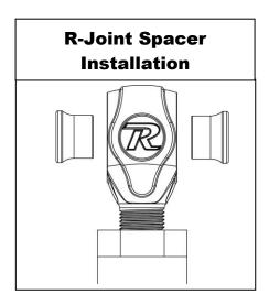
New R-Joints will be quite stiff (75-90 in/lbs breakaway torque) until they "break in" after a few miles of use. After the break in period they will move much more freely. Because the composite bearing race contains self-lubricating ingredients, no additional lubrication is needed or desired. Any additional lubrication will only serve to attract more dirt and debris to the R-Joint and actually shorten its life.
