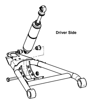
3. Bolt the Shockwave or CoilOver to the lower arm using the supplied 1/2" x 3 1/4" bolt and Nylok. An aluminum spacer on both sides of the eye will center the Shockwave.
