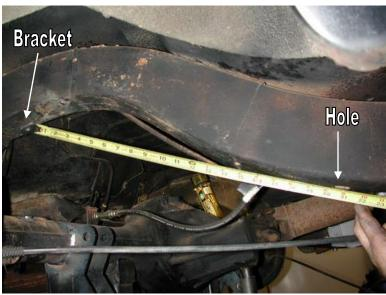
6. The location of the upper Shockwave mount is determined by measuring 20 1/4" from the edge of the bracket to rear edge of the large hole in the bottom of the frame.
