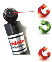
Low speed compression adjustment is used to dial in the handling of your vehicle.
