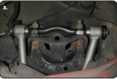
**3.** The Upper Control Arm is attaching the factory mount using factory hardware. Reinstall the shims in the location they were removed from. The passenger side arm is shown in **Figure "3"**.
