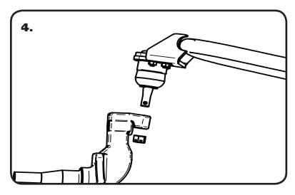
**4.** Attach the Spindle to the control arms. These control arms use a tall ball joint, the boot will NOT touch the spindle. This is normal.
