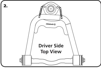
**2.** The Upper Control Arm is attached to the factory frame using factory hardware. The driver side arm is shown in **Figure "2"**. The Ball joint is located on the arm to the REAR of the car.
