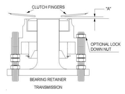
After making sure this is correct and the jam nuts are positioned equally from the transmission mounting surface use the middle jam nut to secure the position of the top jam nut.
