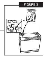
• With battery fully charged and engine running at 1,500rpm, measure
