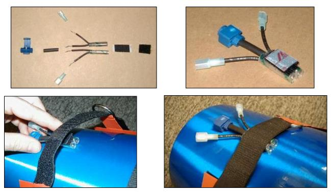
2. Secure the heater element around the bottle with the Velcro straps attached to the heater element.
