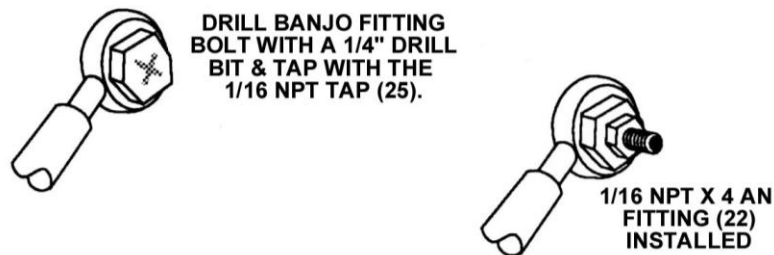
Figure 8 Schematic of "Drilled Out" Banjo Fitting
