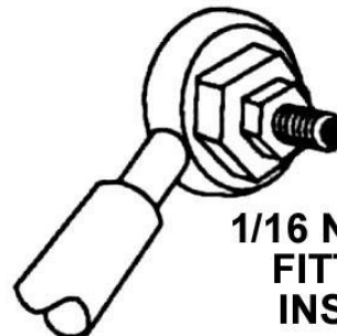
Figure 8 Schematic of "Drilled Out" Banjo Fitting
