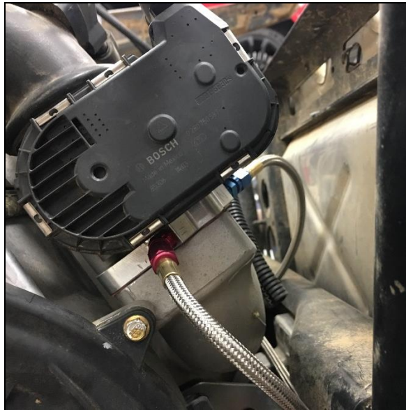
Figure 10 – Installed Nitrous Plate
