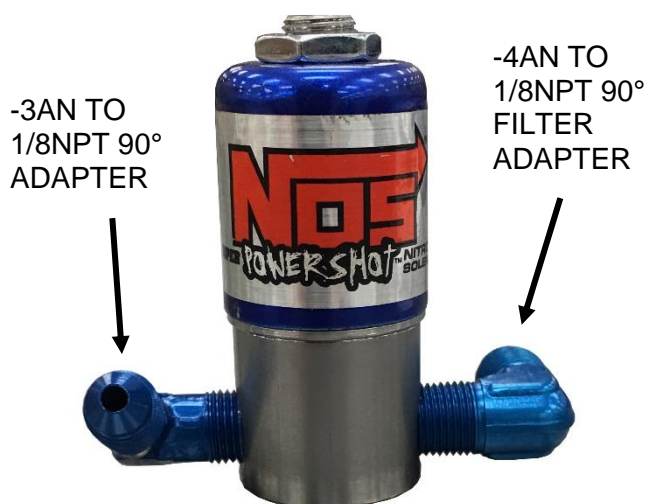
Figure 4 – Nitrous Solenoid Adapter Alignment
