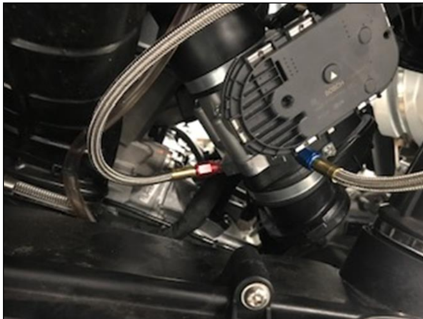
Figure 10 – Nitrous Plate Installation
