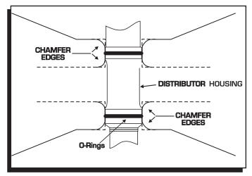
Figure 11 Modified Chevy Block for use with O-Rings.
