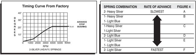
Figure 2 The Factory Equipped Curve.
