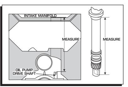
Figure 9 Measuring Oil Pump Shaft Overlap.
