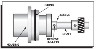
Figure 7 Removing the Retaining Sleeve.
