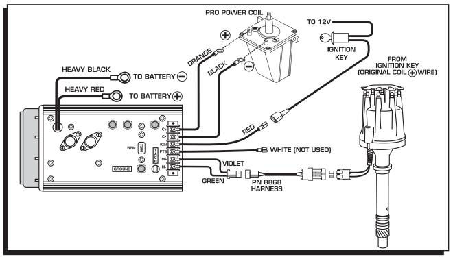
Figure 13 Wiring to an MSD 7ML-2 Ignition Control.
