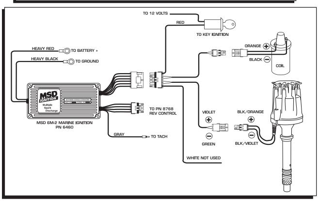
Figure 12 Wiring to an MSD 6M-2 Ignition Control.
