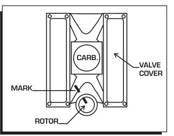
Figure 10 Marking the Rotor Location.
