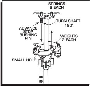
Figure 8 Locking Out the Advance.
