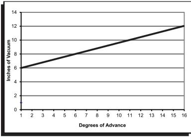
Figure 10 Vacuum Advance and Timing Chart.
