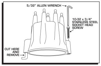
Figure 9 Optional Installation by Bolting Cap Down.
