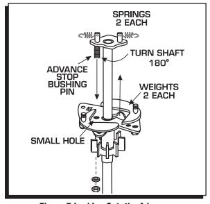
Figure 7 Locking Out the Advance.
