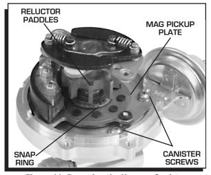
Figure 11 Removing the Vacuum Canister.
