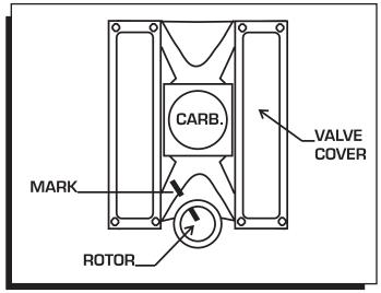
Figure 8 Marking the Rotor Location.
