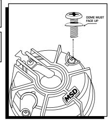
Figure 1 Washer Installation.
