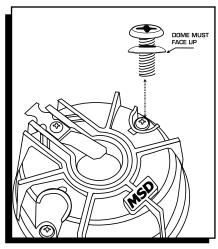
Figure 1 Washer Installation.
