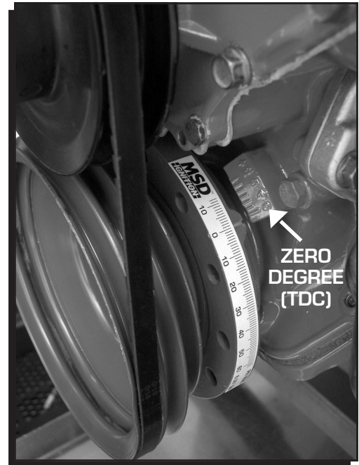
Figure 9 The Timing Tape Installed.
