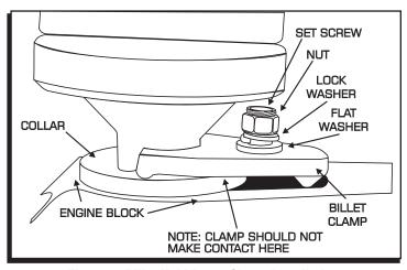
Figure 1 Billet Hold Down Clamp Installation.
