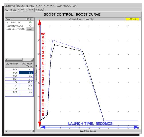
Figure 8 Boost Control: Boost Curve
