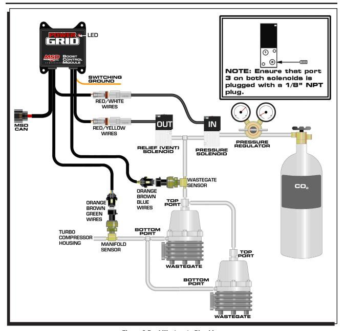
Figure 2 Dual Wastegate Plumbing
