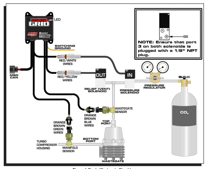
Figure 1 Single Wastegate Plumbing
