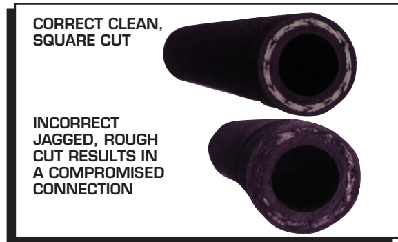
Figure 5 Severing the Hose Properly.
