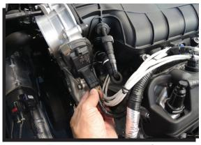
Figure 2 Disconnect the ETC.
