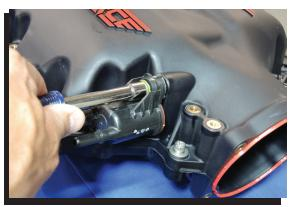
Figure 9 Install the EVAP Solenoid.
