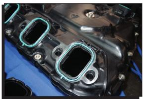
Figure 11 Install the Port Seals.
