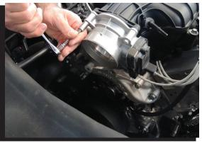
Figure 4 Remove the Throttle Body.
