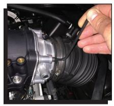
Figure 15 Installing the Throttle Body.
