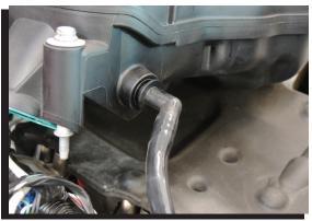
Figure 6 Brake Booster Vacuum Connection.
