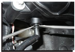
Figure 7 Removing the Brake Booster Tube.
