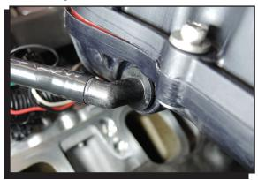
Figure 12 Connect the Brake Booster Tube.
