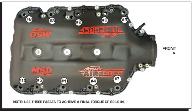
Figure 13 Intake-to-Cylinder Head Torque Sequence.
