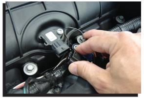
Figure 5 Disconnect the MAP Sensor.
