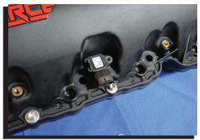
Figure 8 Install the MAP Sensor.
