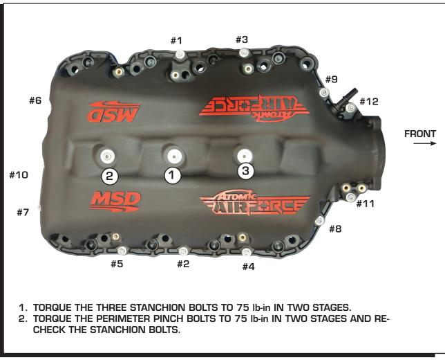
Figure 10 Intake Upper Shell - Torque Pattern.
