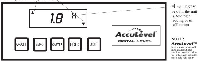
**NOTE:** This Ver. 4 AccuLevel™ has 2 modes of operation. 1) In Normal angle measurement mode the display is steady. 2) In Caster Mode the display flashes (and will not measure absolute angles). Push CASTER button to exit Caster mode and go back to Normal angle measurement.
