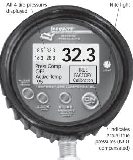
TO TAKE TIRE TEMPERATURES: Push MDD button. Display will change as shown. Take temps as you normally would. Insert the probe into the tire to the same depth each time, on the outside edge, the center, then inside edge.
