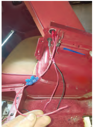
20. Install terminal (11) to red wire (7) then plug it into on/off switch reaming post. Then use fuse holder (10) and more red wire (6) to reach power source.
