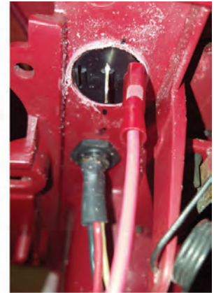
19. Install terminal (11) on momentary switch red wire then plug it into On/Off switch.
