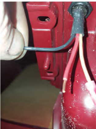
18. Extend momentary switch black ground wire with splice (13) , black wire (5) and eyelet (12) . Ground this wire to chassis (this kit was grounded at firewall).
