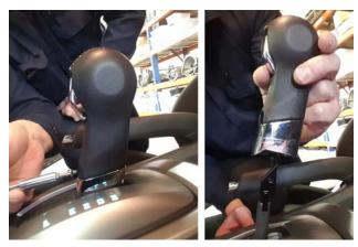
3. Remove screw from front of shifter handle then remove handle.
