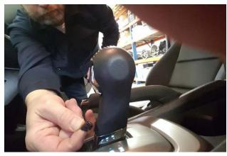
2. Remove screw cover from front of factory shifter.
