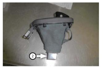
Slide boot up pistol grip base as far as it will go. Then apply a small drop of thread locking fluid to set screw (2) threads and start it in pistol grip.
