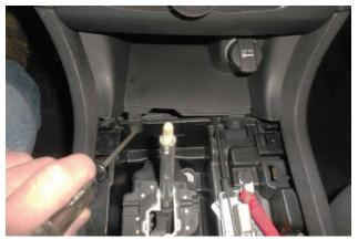
NOTE: Challenger models do not require this step.11. Remove screws (x2) from front console storage tray.
