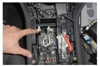
Route harness to driver side of shifter housing. Place stock handle into empty space in front of shifter housing under tray (removed step 11). Challenger models have an empty space just forward of shifter housing.
