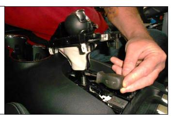
4. Remove the two Phillips screws then pull up on the shift handle to remove it.
