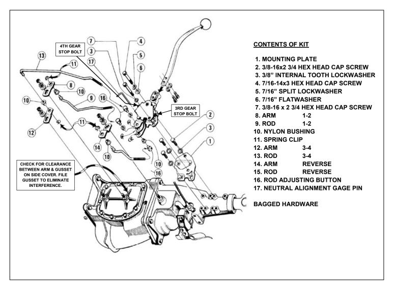
MOUNT SHIFTER IN FORWARD POSITION. THE RODS SUPPLIED WITH THESE KITS ARE DESIGNED FOR <u>FORWARD</u> MOUNTING.
