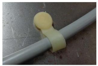
10. Secure cable to chassis using clamps (x2) (3). Drill  $\frac{1}{2}$ " hole in tunnel or frame, fold clamp around cable and push split end through the  $\frac{1}{2}$ " hole. Push pointed end into split end until it snaps tight.
