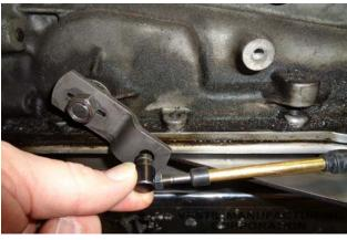
13. Thread cable pivot (6) onto threaded end of cable.
