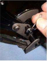
6. Engage first gear, all the way back, then slide cable eyelet over pin on shifter stick. Install **cotter pin (5)** through hole in shifter pin to hold cable in place.
