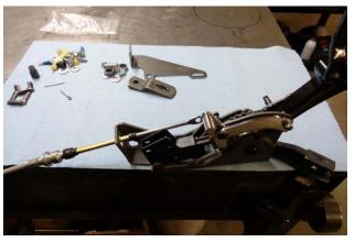
4. With shifter mounted in desired location, direct eyelet end of **shifter cable (2)** through shifter frame.
