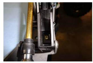
19. Plug female connectors onto spade terminals of micro switch located in plastic switch housing.
