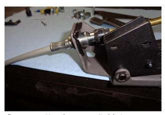
5. Secure cable to frame using **clip (4)**, then press down until it is firmly seated.
