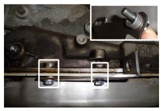
NOTE: If the transmission on your vehicle has an aluminum pan, do NOT use spacers.
