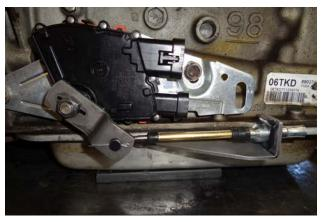
14. Make sure transmission is in first gear (fully back), then thread cable pivot in or out on cable until it lines up directly with hole in transmission arm. Insert cable pivot into hole in transmission arm.
