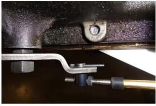
16. When satisfied with adjustment, secure cable pivot to transmission arm using supplied **cotter pin (11)**. Lock cable pivot in this position with 10-32 nut supplied on shifter cable.
