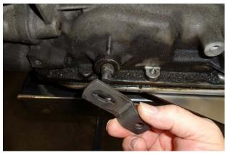
11. Install transmission arm (12) as shown.
