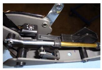
NOTE: If necessary, loosen screw on adjusting collar located near shifter handle then adjust slide mechanism back and forth until vehicle starts in neutral and park only.
