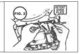
Loosen screw that fastens the extension spring anchor plate to release tension on the detent roller.
