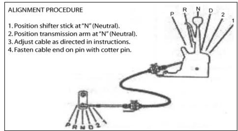
With shifter mounted in the desired location, direct eyelet end of shifter cable through shifter frame. Secure shifter cable to frame using cable clip, push clip down until it is firmly seated. Put shifter in neutral and slide cable eyelet over pin on shifter stick (see exploded view), install cotter pin (p/n 1900001) through hole in shifter pin to hold cable in place.
