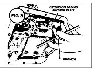
Loosen the socket head cap screw that fastens the throttle pressure actuator (transmissions that have throttle pressure control).
