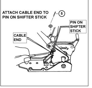
**WARNING!** Installation of Quarter Stick shifter on Powerglide transmission eliminates throttle pressure control linkage (kickdown valve).
