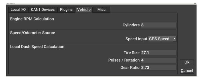
GPS Speed: Use this setting with the internal GPS. No additional setup is required.
