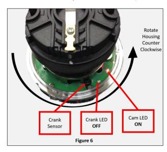
Slowly turn the housing <u>counter-clockwise</u> until the Crank LED goes **OFF** (Figure 6).
