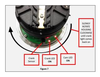
Turn the housing **clockwise** until the Crank LED comes back **ON** (**Figure 7**). Stop at this point. This will position the distributor close to where it needs to be. Install and snug the distributor clamp down at this point.
