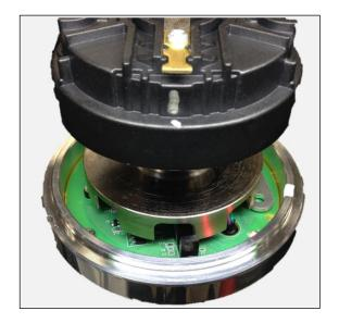
The relationship between the crank sensor, shutter wheel opening, and rotor in the picture above should match what is installed in your engine.
