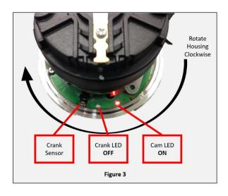
Slowly turn the housing <u>clockwise</u> until the Crank LED goes **OFF** (**Figure 3**).
