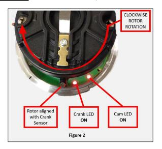
For engines that have the rotor rotating **clockwise**, turn the housing until the rotor contact is pointed at the black crank position sensor (**Figure 2**). Both the cam and crank LED should be illuminated **(ON)**.
