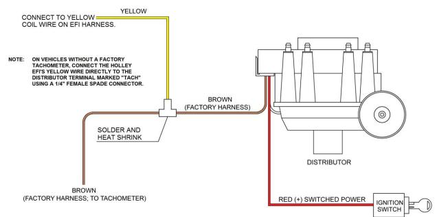
Figure 26 below shows how to connect to a factory style ignition with a canister style coil.
