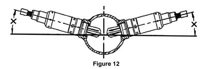
**NOTE:** The oxygen sensor should be mounted in such a way that the condensation in the exhaust tubing will not enter the sensor. Mount the O<sup>2</sup> sensor in the upper half of the exhaust tubing, with the angle "x", shown above, being greater than 10°. The picture above indicates that the sensor can be mounted on either side of the exhaust tubing.
