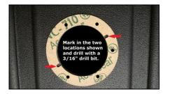
*Figure 1*: Gasket being used as template to mark drilling locations
