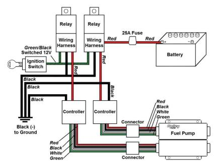
Holley BLDC (Brushless DC Controller) Introduction and Setup
