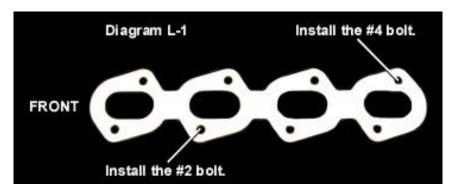
**NOTE:** Some header flange bolt holes are slotted for the ease of bolt installation and are not intended to be installed before the header is inserted into the engine bay. Only the bolts specified in the installation procedure should be installed before the header is inserted into the engine bay.
