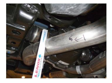
7. Unbolt hangers (x2) behind rear differential from cross member. Slide muffler assemblies forward and out of hanger mounts, leaving front hangers attached. Deburr pipe ends then index and remove hanger mounts (x2).
