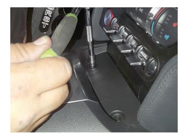
30. Reinstall bolts (x2 ea.) then left and right kick panels (removed step 18).
