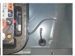
16. Pull enough of wire assembly up through access point to reach front of vehicle. Route it under carpet to front passenger corner of trunk and push it through into vehicle cab.
