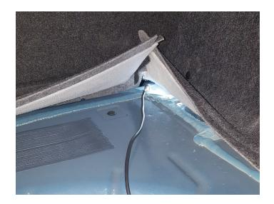
17. Lift rear seat, pull wire outside of seat bracket and belt then follow wiring harness.
