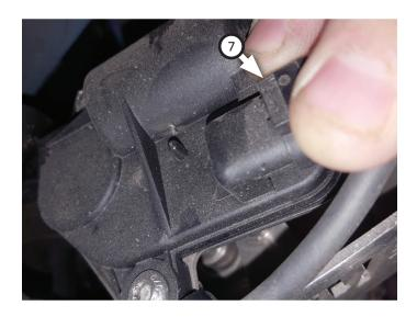
15. Open trunk and remove spare tire cover. Cut slit or "x" in access point, apply lubricant to opening then push wire connector through it.
