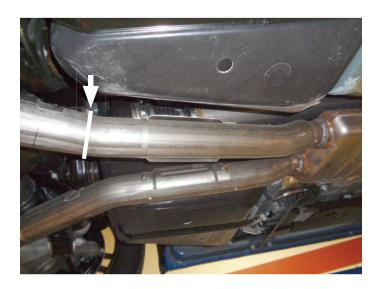
**NOTE:** Use caution as you cut pipes to avoid cutting other engine components.
