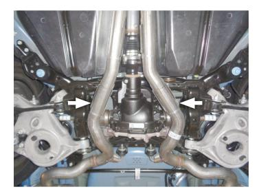
5. Mark each pipe just behind second bend (where bend straightens out). Unplug factory exhaust actuator then tuck connection up and away. Cut tailpipes at muffler exits, disassemble hanger wires and remove them.
