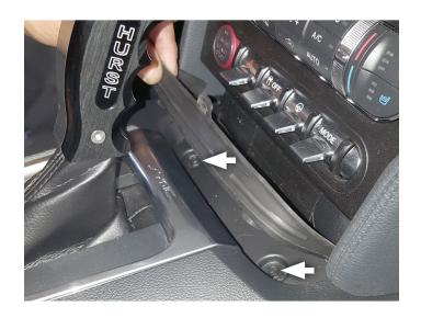
20. Lift mat inside console and remove and retain nuts (x2). Lift top portion of center console from lower portion. Find something that can block top portion up so you can work under it in following steps.
