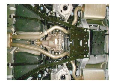
4. Remove heatshields by cutting through rear strap. Lift and lower them a few times to break weld at front then remove shield.
