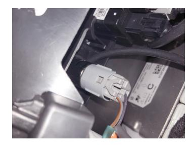
23. Carefully strip factory loom back from plug. Using a test meter or light, turn ignition to "ON" then identify power feed and ground wires.
