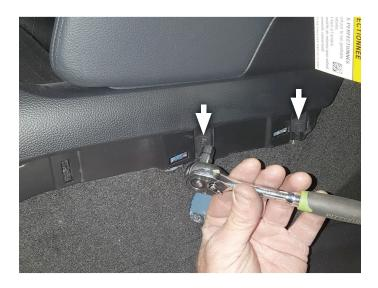
19. Remove screws (x2) under center console forward storage tray. Retain them for later use.
