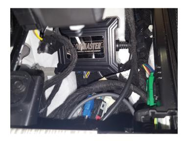
28. Plug in connecter (from step 22) then replace top portion of center console back onto lower portion.
