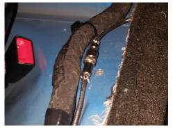
22. Locate center console rear power outlet and unplug connector.
