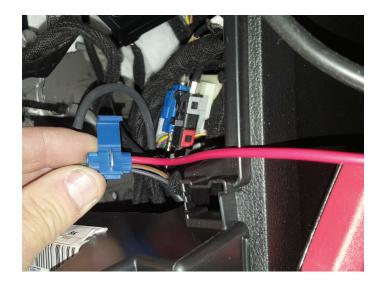
27. Install **fuse (13)** into fuse holder then test operation of valves. Secure controller kit module in center console where convenient.
