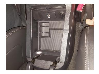
29. Reinstall center console forward storage tray with bolts (x2) (removed step 19).
