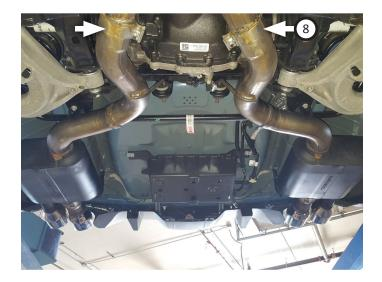
14. Plug wire assembly (7) connector ends into left and right muffler actuator motors.
