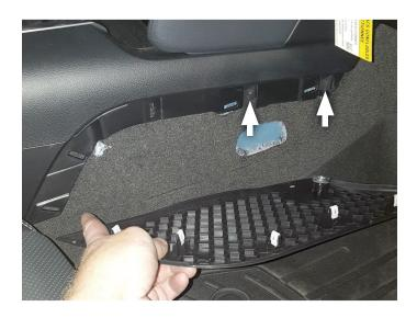
31. Replace rear seats and any loose flooring. Then install spare trunk cover. As you do, secure wire slack so it wont get damaged and stays in place, using zip ties as necessary.
