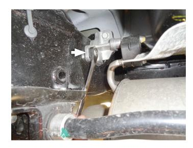
4. Remove upper bolt from left and right rear mounts, disassemble hangers from isolators and remove muffler from inlet pipe. Transfer driver side hanger mount onto new tailpipe.
