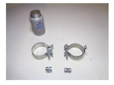
6. Place **clamp (2)** onto **tailpipe (1)** and connect it to factory over-axle pipe. Line inlet pipe notch up to overaxle pipe tab but don't cover notch. Tighten clamp just enough to allow for further adjustment.
