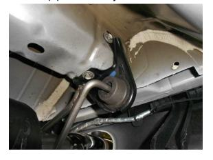
4. Loosen the four nuts at the two band clamp connections at the inlet of the center resonator. Using a screwdriver, pry up the clips on the clamp body to release the clip from the tab on the inlet pipes. Slide the clamp assemblies slightly back to clear the tabs. With the help of an assistant, carefully lower the stand and slide the assembly back to disengage from the inlet pipes.
