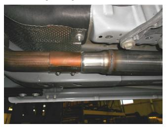
2. Place the inlets of the axle-back muffler assemblies onto the back of the Flowmaster X-Pipe, be sure to slide them fully on and tighten the clamps enough to hold but still allow for adjustment. See steps 4 and 5 on page 5 for final adjustment steps.
