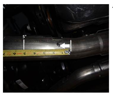
4. Measure back 5" from the beginning of the straight area marked in the previous step and make a mark on both pipes as shown in the photo at left. Support the exhaust system both in front and behind the area to be cut. Check that the marks are correct, then using a sawsall, cut both pipes at the marks. Note: Due to the closeness of the pipes to the gas tank, use caution when cutting! Carefully deburr the end of the muffler inlet pipes where cut with a file or die grinder.
