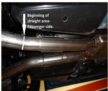
3. Behind the factory center resonator, follow the pipes back just past the second bend of each pipe, make a mark on each pipe where the bend ends and the straight area begins. See above photos.
