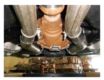
2. Place a stand under the center resonator just forward of the axle-back muffler assemblies. Loosen the clamps at the inlets of the Flowmaster axle-back mufflers.
