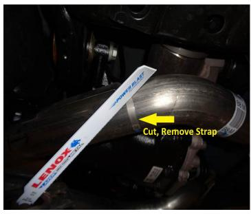
2. Begin by removing the two pipe heatshields indicated in the first picture above. Cut thru the strap at the rear of the shield, then lift and lower the shield a few times to break the weld at the front of the shield. Remove.
