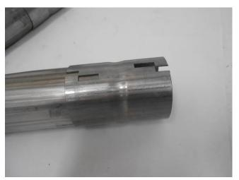
Slide the supplied TB809S adapter pipes onto the end of each outlet of the 86480S X-pipe assembly. Place a supplied clamp onto the connections and tighten enough to hold.
