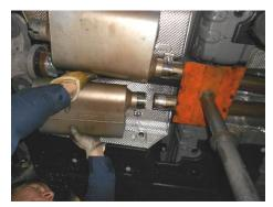
5) Place a supplied 2  $\frac{1}{2}$ " clamp onto the inlet of each #842546-**Z** muffler. Then fully slide the mufflers onto the back of the Scavenger pipe assembly and support with stands. Level the mufflers and tighten the clamps enough to hold, but still allow for adjustment.
