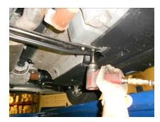
2) Using a 13mm socket, unbolt the two body braces in the center of the vehicle. The braces will be re-installed after completing step 2 of the installation instructions below.
