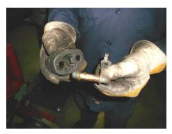
3) To install the new Flowmaster system you will need to remove the factory hanger located on the cross member just behind the rear differential. After unbolting the hanger, remove the rubber isolator from the hanger mount, the rubber isolator and the bolt/washer securing the hanger will be reused with the Flowmaster system.
