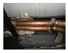
2) Begin by placing a supplied 2  $\frac{1}{4}$ " clamp onto each of the slip fits on Scavenger pipe #86331S. Place the Scavenger pipe onto the back of the stock head pipes (make sure the Flowmaster embossing is facing the ground). Level and center the assembly in the drive line tunnel and support with a stand. Tighten the two clamps enough to hold, but still allow for adjustment. Reinstall the two body braces onto the vehicle and tighten securely.
