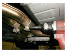
3) Support the rear of the system with a stand. Then starting at the rear of the vehicle, remove the hangers on the system from the rubber mounts on the vehicle, also un-clip the ground strap from the middle hanger on the right tailpipe. Then using a 15mm socket, loosen the clamps at the slip fit connections behind the catalytic converters and with the help of an assistant, lower the stand and slide the system back off of the head pipes. Carefully lower from the vehicle.
