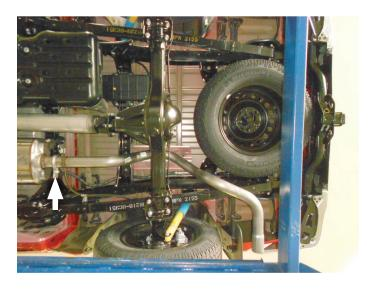
Remove bolts (x4) from front flange connections. Disassemble wire hangers from isolators then remove muffler assembly from vehicle. Retain bolts for later use.
