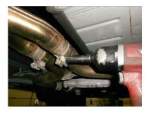
Support the rear of the system with a stand. Starting at the rear of the vehicle, remove the three hangers on the right side of the system from the rubber mounts on the vehicle. Unclip the ground strap from the middle hanger on the right tailpipe and using a 15mm socket, loosen the clamps at the slip fit connections behind the catalytic converters. Then with the help of an assistant, lower the stand and slide the system back off of the head pipes. Carefully lower from the vehicle.
