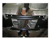
1) Raise the vehicle and support securely with stands. To ease the removal of the stock system, spray a penetrating lubricant onto all of the rubber hangers of the system. Use a 13mm socket to loosen the six nuts attaching the two factory body braces to the underside of the vehicle, set the braces aside for re-installation in step 4 below.
