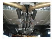
4) Begin by placing a supplied 2¼" clamp onto each of the slip-fits of Scavenger pipe **#16705S.** Then place the Scavenger pipe onto the back of the stock head pipes (make sure the Flowmaster embossing is facing the ground). Level and center the assembly in the drive line tunnel and support with a stand. Tighten the two clamps enough to hold, but still allow for adjustment. Reinstall the two factory body braces removed in Step 1 above and tighten securely.
