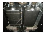
5) Place a supplied 2½" clamp onto the inlet of each muffler **#842551-Z.** Then fully slide the mufflers onto the back of the Scavenger pipe assembly and support with stands. Level the mufflers and tighten the clamps enough to hold, but still allow for adjustment.
