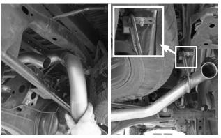
13. Slip a clamp (11) over the right over-axle pipe. Install the universal bracket (12) on the right tail pipe's (6) hanger rod, with the flat pointing outboard and facing up toward the frame. Slip the tail pipe over the over-axle pipe. Then fasten the bracket to the frame with the bolt (13) and a flat washer (15) against the frame, and the other flat washer (15), the lock washer (16), and the nut (14) against the bracket. Verify 3" of insertion, and snug the clamp slightly.
