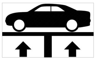
**1. Raise the vehicle** to working height on a lift. If you do not have a lift, securely support the vehicle on jack stands.
