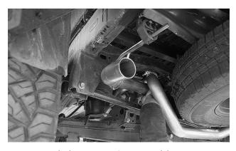
**14. Slip a clamp (11) over the left tail pipe (7).** Install its hanger rod in the rubber isolator, then slip it over the over-axle pipe. Verify 3" of insertion, and snug the clamp slightly.
