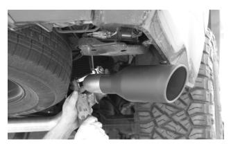
**16. Install a tip (10) on each exit pipe.** Align each tip as desired, and tighten its clamp.
