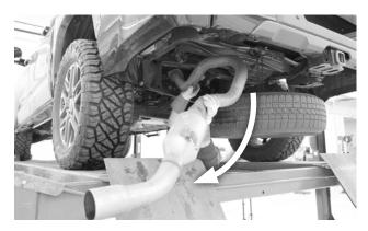
**3.** Lower the spare tire for clearance, and remove the tailpipe from the vehicle.
