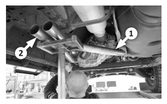
**7.** Attach left (2) and right (1) inlet pipes to factory exhaust with the 2 stock gaskets, and 4 screws and springs, ensuring that both pipes are oriented properly.
