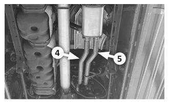
12. Slip a clamp (11) over the muffler's left outlet. Move the left over-axle pipe (5) into place, and insert its hanger rod into the rubber isolator. Insert the pipe into the muffler, verify 2" of insertion, and snug the clamp slightly. Repeat the process for the right over-axle pipe (4).
