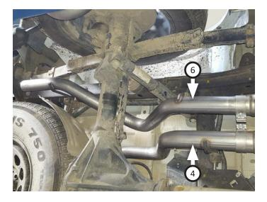
11. Place 2-1/2" clamp (12) onto left rear tailpipe (5) then connect it to left front tailpipe. Insert wire hanger into rubber hanger then tighten clamp enough to hold parts.
