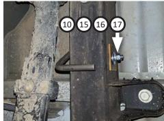
Route left front (4) and right tailpipes (6) over axle then connect them to muffler. Insert their wire hangers into isolators then tighten clamps just enough to allow for adjustment.
