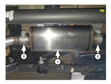
10. Route **overaxle pipe (4)** over axle then connect it to muffler. Insert wire hangers into isolators then tighten clamp just enough to allow for adjustment.
