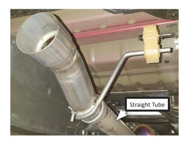
9. Place (x2) clamps (8) onto muffler (3) then connect it to inlet pipe. Tighten clamp just enough to allow for adjustment.
