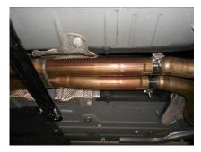
2) Begin by placing a supplied 2 ½" clamp onto each of the slip fits on Scavenger pipe **#86337M.** Place the Scavenger pipe onto the back of the stock head pipes (make sure the Flowmaster embossing is facing the ground). Level and center the assembly in the drive line tunnel and support with a stand. Tighten the two clamps enough to hold, but still allow for adjustment. Reinstall the two body braces onto the vehicle and tighten securely.
