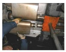
3) Place a supplied 2 ½" clamp onto the inlet of each **#71226-Z** muffler. Then fully slide the mufflers onto the back of the Scavenger pipe assembly and support with stands. Level the mufflers and tighten the clamps enough to hold, but still allow for adjustment.
