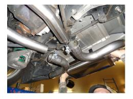
8. Place a provided clamp onto the inlets of muffler **7525554-470**. Place the muffler up into position and slide onto the intermediate pipes, make sure they are fully seated and support the muffler with a stand. Tighten the clamps enough to hold but still allow for adjustment. Place a provided clamp onto each muffler outlet. **NOTE:** The protective plastic wrap has been left on the muffler to protect the finish; **remove it prior to starting the vehicle.**
