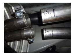
5. Place the left inlet pipe **#86424M** into position behind the left catalytic converter and re-install the nuts removed in step 2 above. Tighten enough to hold but still allow for adjustment. Be sure to replace the gasket. Repeat the step on the right side of the vehicle with inlet pipe **#86423M**. Measure and make a mark at 1-3/4" from the back of each of the front pipes, this is the mark that the X-pipe will be slid on to.
