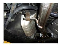
7. Place the left intermediate pipe **#86426M** into position and slide into the back of the X-pipe, connecting the hanger on the pipe to the rubber mount on the vehicle. The hanger should be level and the rubber isolator should be vertical. Repeat the step on the right side of the vehicle with pipe **#86427M**. Tighten the clamps enough to hold but still allow for adjustment.
