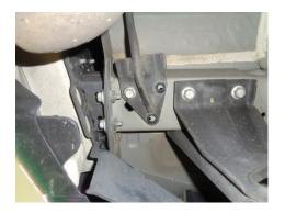
4. At the rear of the muffler, remove the three bolts securing the two rearmost hangers to the frame of the vehicle. Lower the stand and slide the system down and to the rear to remove from the vehicle.
