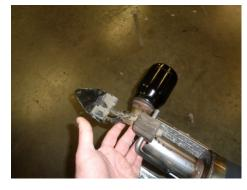
9. Place the new exit pipe assemblies **86430M** & **86431M** next to the factory muffler and swap the right and left rear hangers to the new exit pipes.
