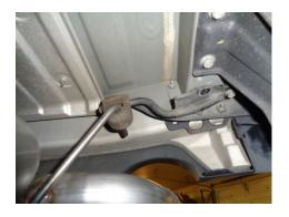
10. Place the left exit pipe **#86430M** into the left muffler outlet and re-install the factory hanger mount to the frame using the factory bolts, tighten securely. Adjust the tip to the desired position and tighten the clamp enough to hold, but still allow for adjustment. Repeat this step on the right side of the vehicle with exit pipe **#86431M**.
