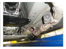
2. Remove the nuts at the two flanged connections behind the catalytic converters, then remove the nuts at the flanged connection in the center of the vehicle. Slide the Y-pipe rearward to disengage the front two flanges, then lower the front of the Y-pipe and disengage the center connection. Lower from the vehicle and set aside. Save the front two gaskets for reuse.
