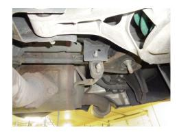
3. Support the rear muffler with a stand; disengage the two middle hangers and the hanger at the front left corner of the muffler from the rubber mounts on the vehicle.
